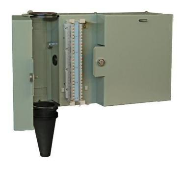
The use of splice chambers allows for the BET's to be mounted closer together, both vertically and horizontally. Large OSP cables can be hidden, resulting in a more aesthetically pleasing and space-saving installation.
