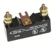
All station protectors come with an external fail-safe mechanism that ensures safe operation even under the most adverse conditions. Under continuous surge conditions, the device will short both sides of the circuit to ground.
